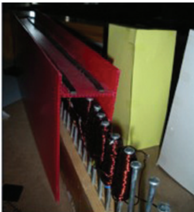
FIGURE 10: ARRAY OF ELECTROMAGNETS IS PLACED UNDER THE RAIL TRACK
