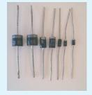
**Diode** is one of the components of a circuit. It consists of two semiconductors. Diode lets the current flow in a circuit only one way. Namely, it is a good conductor only for a certain direction of the current, that's why it is said that it creates some sort of "one way road" in a circuit.
